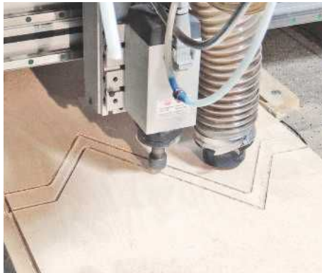
▲ Pic.8 How to cut the zigzag top? "I considered clamping a fence parallel to each line and cutting to it with a handheld router. It would have worked, but would have taken all afternoon and been a nervous operation. Instead I took the opportunity to try out a CNC (Computer Numerical Control) cutting service. Next time I'll want to take my own file on a memory stick, but this time the operator converted my drawing for me. As with sawing up the sheet, precise measurements are essential. The machine passed and re-passed, working to a tolerance of 50 microns (2 thou) which is rather better than I would have managed on that nervous afternoon. Only for the sake of the photograph is the dust extractor hood disconnected.
